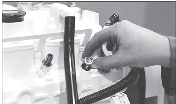
Figure 16: Remove and replace copper sealing washer.
