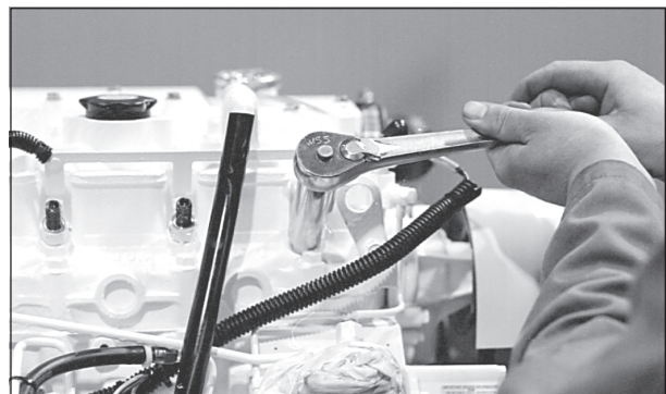
Figure 17: Reinstall injector. Torque to proper tightness.
