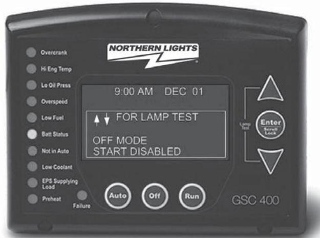
2. AUTO Mode - When the GSC400 is set to the Auto Mode, automatic starting will be enabled. Possible triggers include start/stop, battery recharge and exerciser features (all of which are controllable from the menu system). If the engine is started, failures will be automatically detected allowing for safe engine operation.
