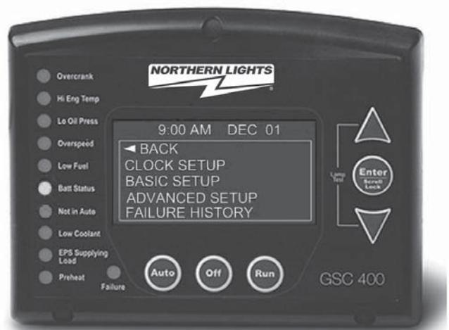
Each menu has a “Back” selection. Scroll up to the Back selection and press the Enter button to go back to the previous menu. When in the basic menu you can go back to the Off state by pressing the OFF key.
