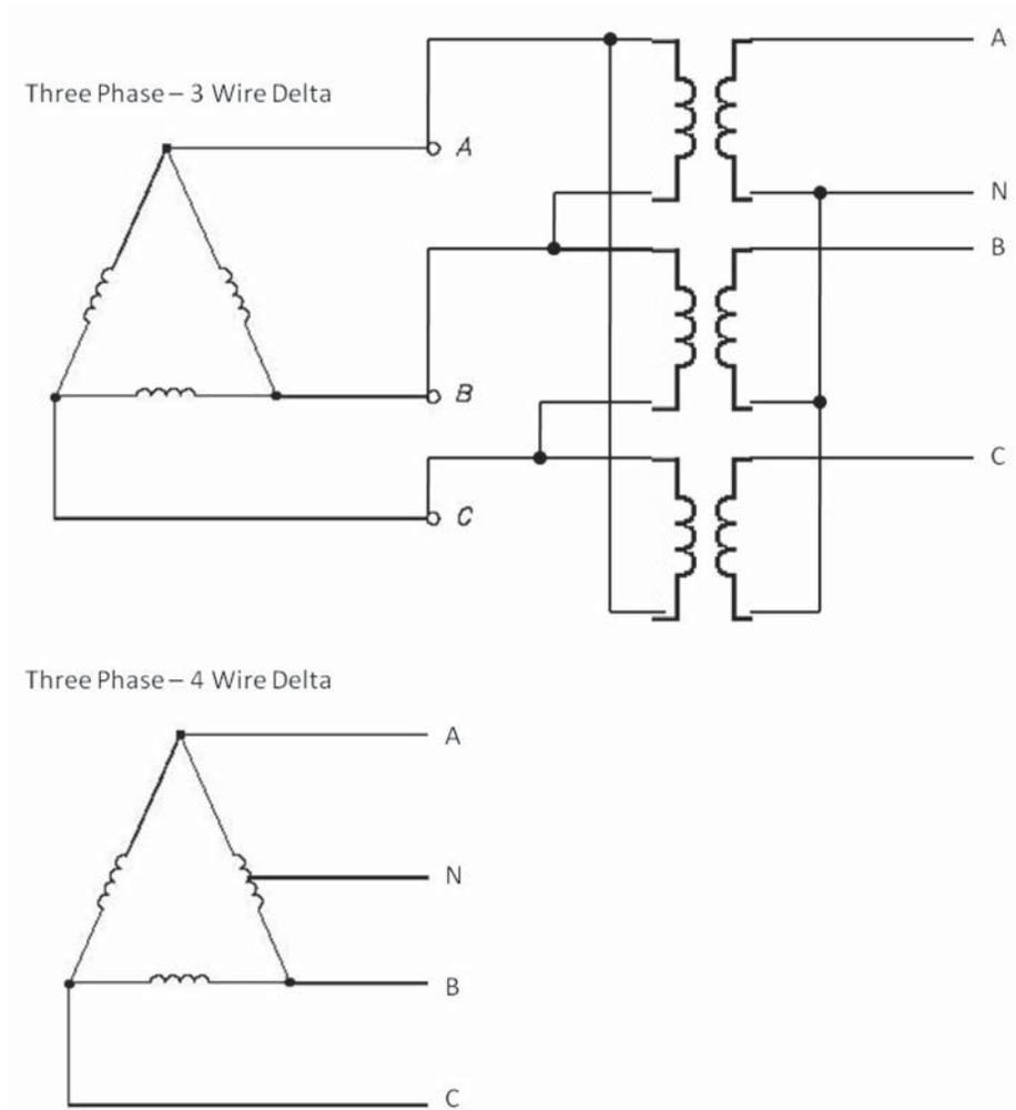
**Figure 6 – Three-wire versus four wire delta generator configurations**
