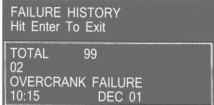
A total of the most recent 100 event/failure conditions will be recorded within the log. Event/failure conditions may be viewed simply by scrolling up or down throughout the menu. In addition to the event/failure condition information, the associated date and time of the event/failure will be displayed.
