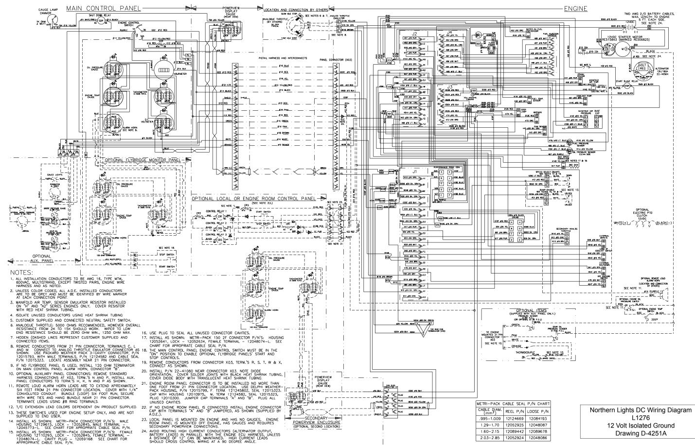
INSTALL AS SHOWN: METRI-FACK CONNECTOR P/N'S: FEMALE HOUSING 12110293, LOCK - 12052845, FEMALE TERMINAL -12048074-L. CAVITY PLUG - 12059168. SEE CHART FOR APPROPRIATE CABLE SEAL P/N.
