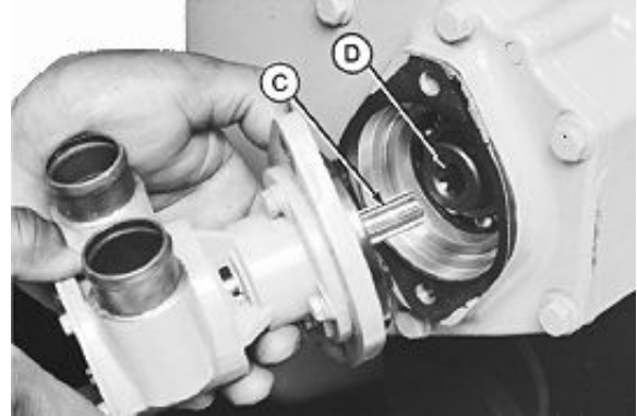
Install Sea Water Pump
