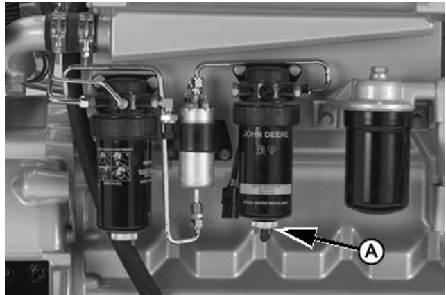
Drain Primary Fuel Filter - 6068SFM50 Shown
