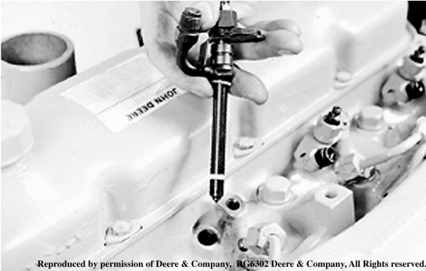
Figure 16: Shows relationship of parts required for installation.
