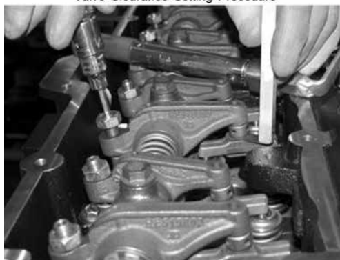
Checking Valve Clearance Using Bent Feeler Gauge
