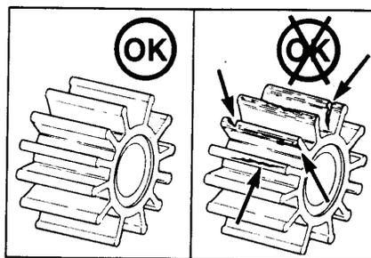
Inspect Pump Impeller
