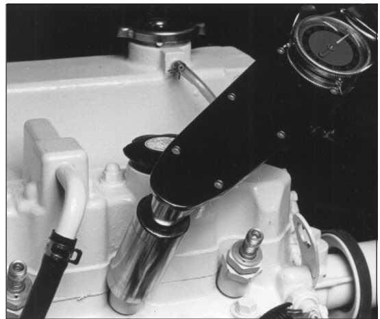
Figure 16: Reinstall injector. Torque to proper tightness.
