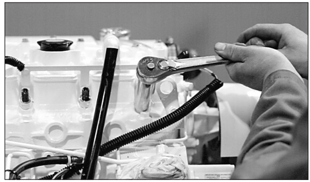
Figure 17: Reinstall injector. Torque to proper tightness.
