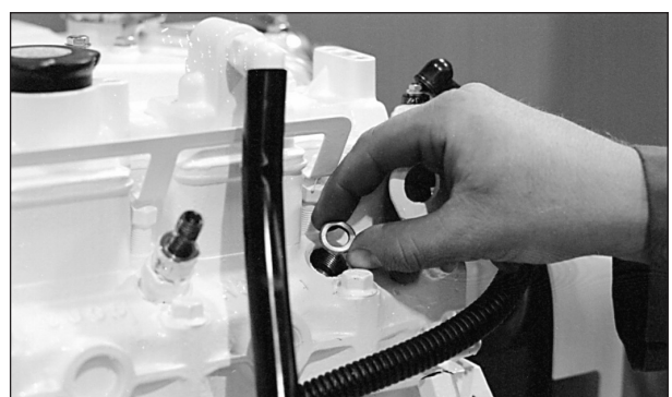
Figure 16: Remove and replace copper sealing washer.
