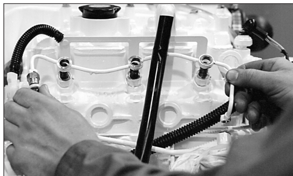
Figure 15: Remove return line.
