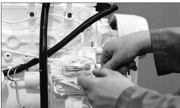
Figure 13: Cover lines, inlets and injection pump outlets.
