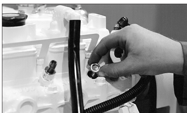
Figure 17: Remove and replace copper sealing washer.
