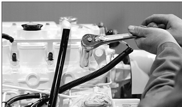
Figure 18: Reinstall injector. Torque to proper tightness.
