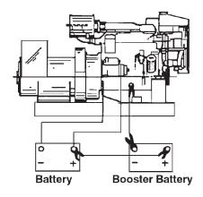
Figure 18: Booster Battery Connections
