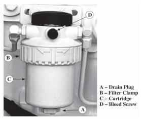
Figure 6: Secondary Fuel filter
