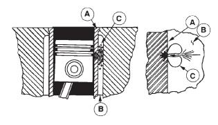
A - Cylinder Liner Walls B - Engine Coolant C - Vapor Bubbles Figure 17.
