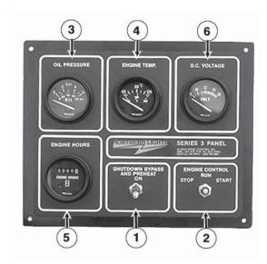
Figure 4-A: Series 3 Generator Control Panel
