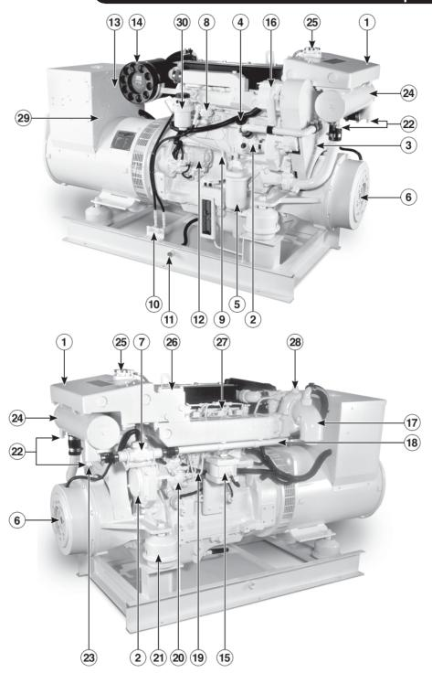
Figure 2: MP445H (note: MP445T models have similar component locations).
