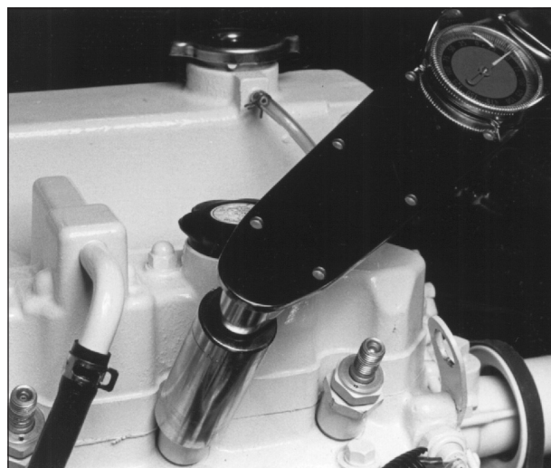
Figure 14: Reinstall injector. Torque to proper tightness.
