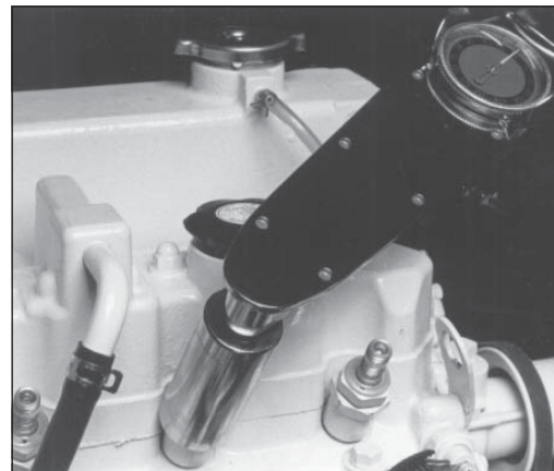
Figure 13: Reinstall injector. Torque to proper tightness.
