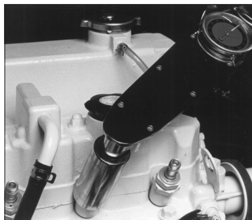
Figure 13: Reinstall injector. Torque to proper tightness.
