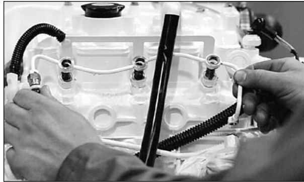
Figure 14: Remove return line.
