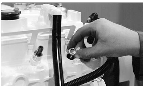
Figure 16: Remove and replace copper sealing washer.
