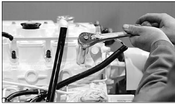
Figure 17: Reinstall injector. Torque to proper tightness.
