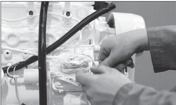
Figure 12: Cover lines, inlets and injection pump outlets.
