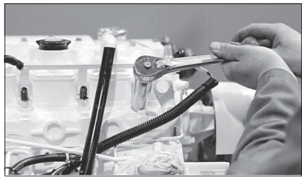
Figure 17: Reinstall injector. Torque to proper tightness.
