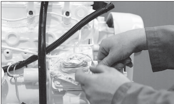
Figure 12: Cover lines, inlets and injection pump outlets.
