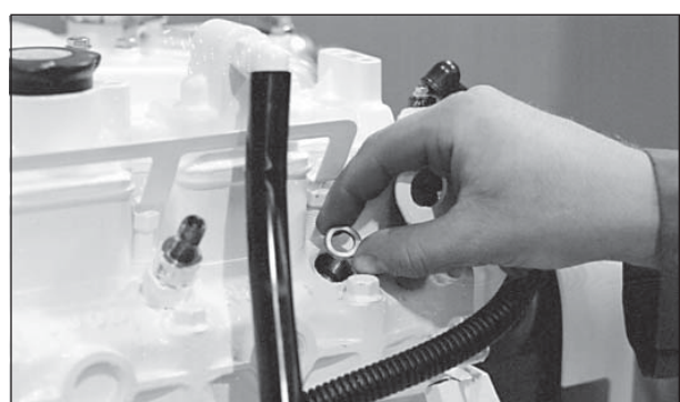
Figure 16: Remove and replace copper sealing washer.
