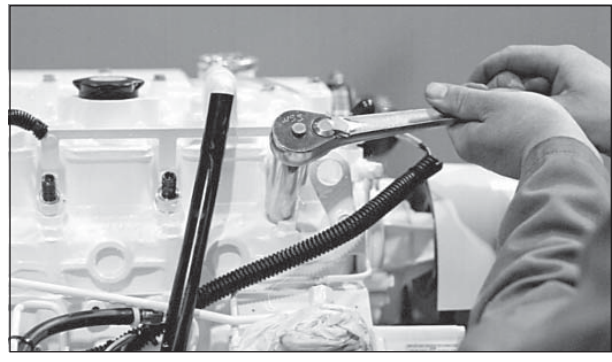
Figure 17: Reinstall injector. Torque to proper tightness.
