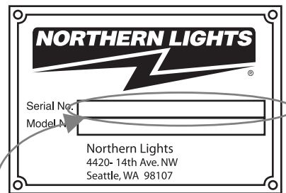
Generator set serial number
