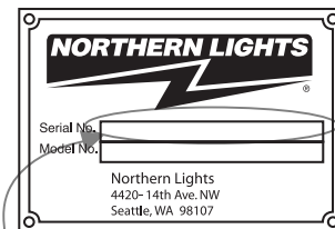
Generator Set Serial Number
