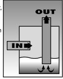
job was done right. Fig. 2: How a water-lift muffler (top) works.
