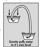
between the pump Fig. 3: Siphon Effect. and the engine's heat exchanger. The top of the loop must be at least one foot above the water line. A siphon break is installed at this point. The siphon break is a small air valve that closes when the pump is working and opens when the pump stops. This forms an air bubble in the loop and makes it impossible for the siphon effect to take place.
