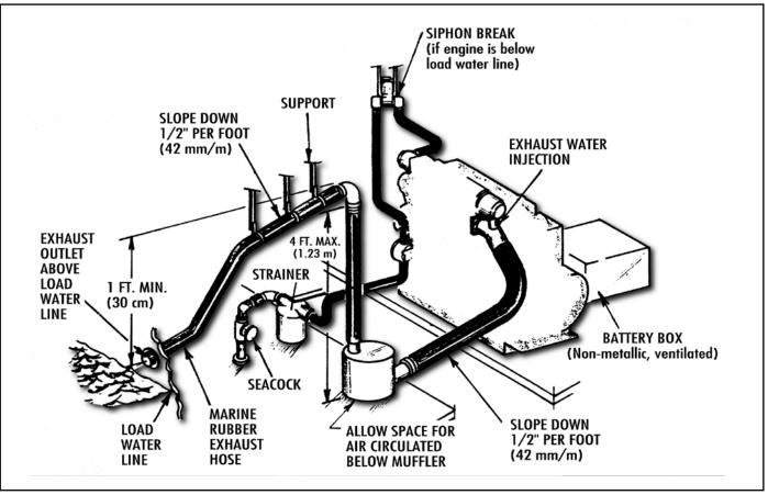
Figure 1. Properly installed wet exhaust system.
