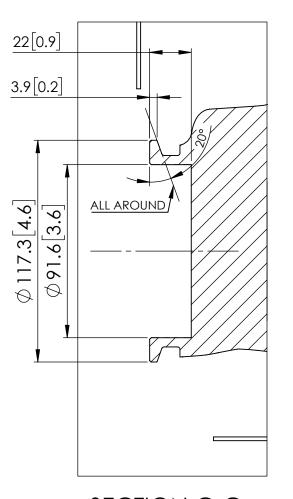
SECTION C-C SCALE 1:2 **EXHAUST CONNECTION** DIMENSIONS
