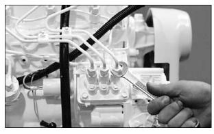
Figure 11: Remove delivery line flare nuts.
