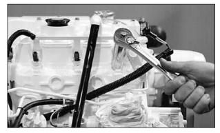
Figure 16: Unscrew injector.
