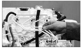
Figure 12: Remove delivery lines.
