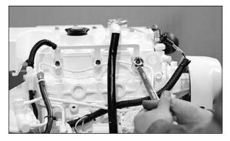
Figure 14: Remove return line nuts.
