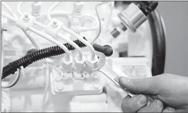
Figure 12: Remove delivery line flare nuts.
