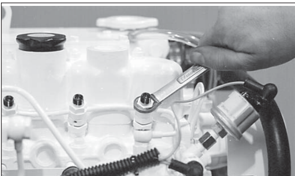
Figure 15: Remove return line nuts.
