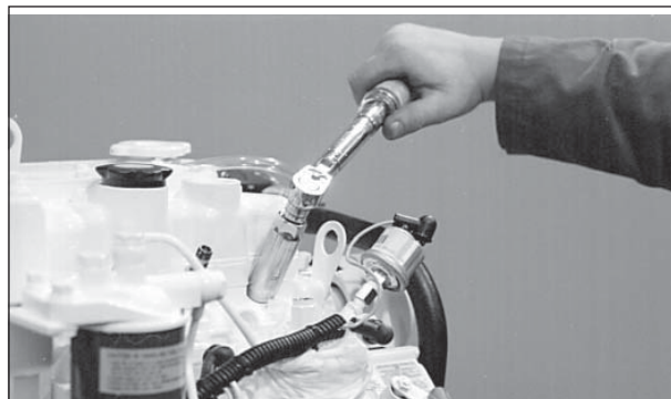
Figure 19: Reinstall injector. Torque to proper tightness.
