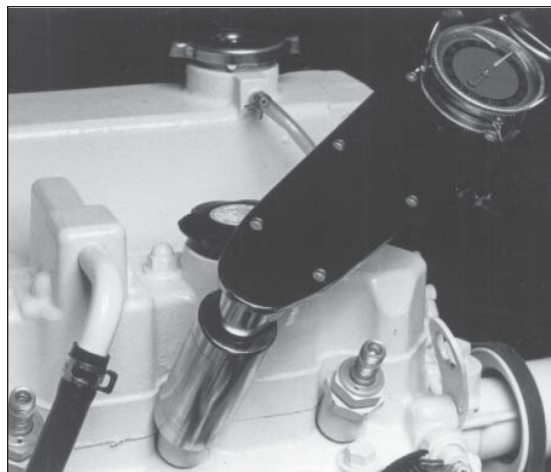
Figure 18: Reinstall injector. Torque to proper tightness.
