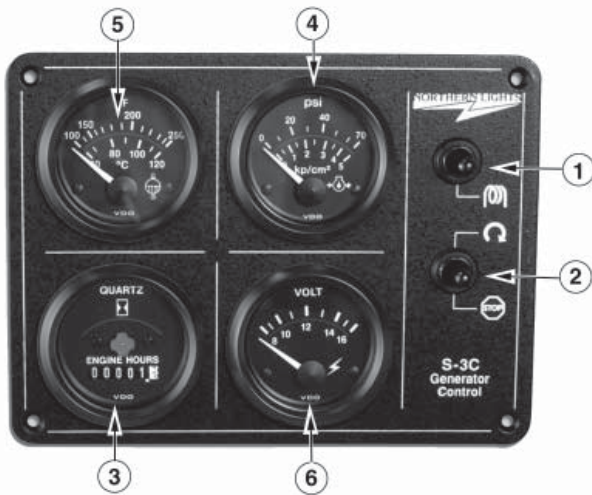
Figure 6-a: Series 3 Generator Control Panel
