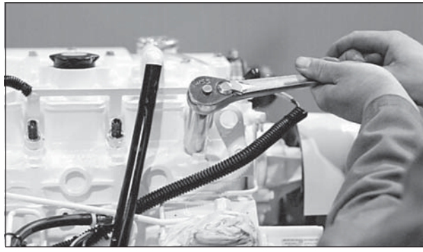
Figure 18: Reinstall injector. Torque to proper tightness.
