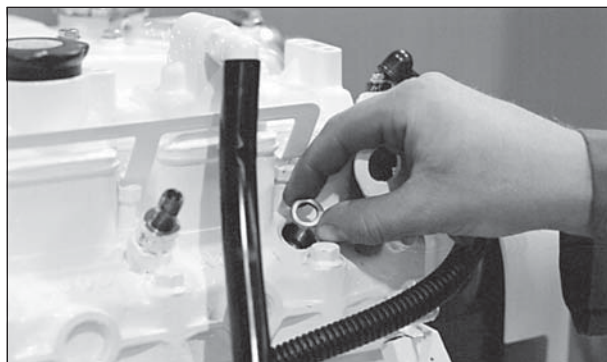
Figure 17: Remove and replace copper sealing washer.
