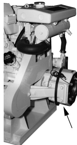
Figure 15: Optional PTO with electric clutch
