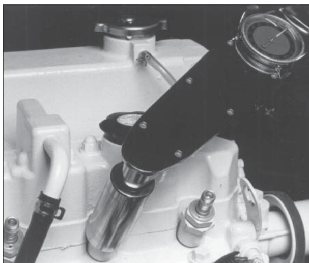
Figure 14: Reinstall injector. Torque to proper tightness.
