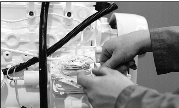
Figure 12: Cover lines, inlets and injection pump outlets.
