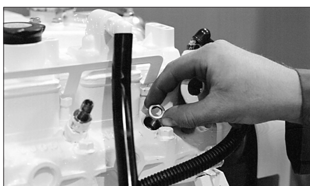
Figure 16: Remove and replace copper sealing washer.
