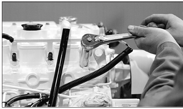
Figure 17: Reinstall injector. Torque to proper tightness.
