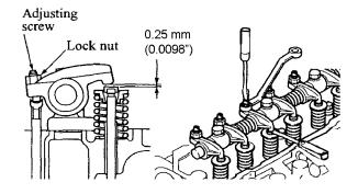
Figure 9: Valve Adjustment
