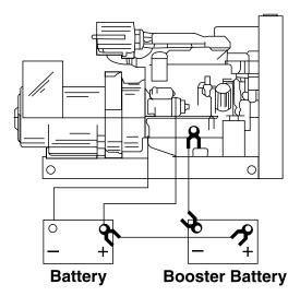
Figure 12: Booster Battery Connections
