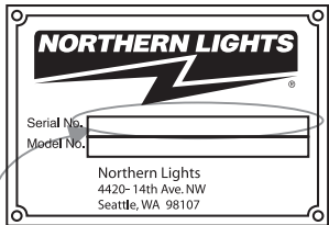
Generator Set Serial Number
