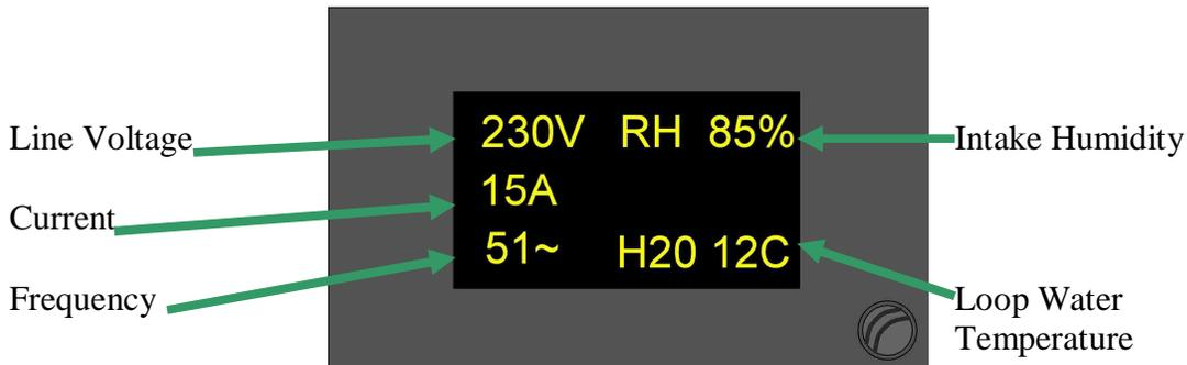
Line voltage, line frequency, system current, inlet humidity, and loop water temperature can be viewed on the display. In the off mode or any operating mode, press and hold either center touch area to view the status. To exit the status view, press and release any touch area on the display.
