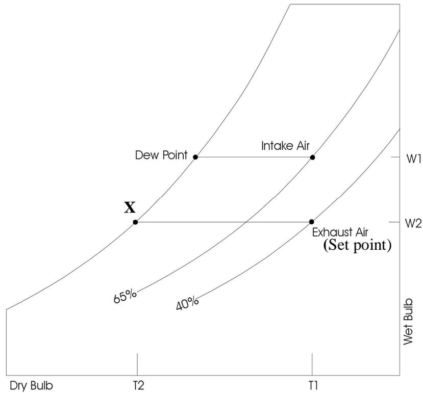
The above graph illustrates the dehumidification process. The intake air temperature is reduced below the dew point. Moisture is removed from the air reducing the dew point and air temperature to point X. The air is then warmed by the electric heater to the set point.
