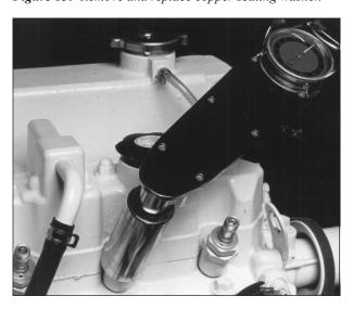
Figure 14: Reinstall injector. Torque to proper tightness.
