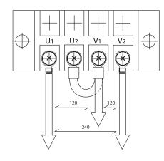
Figure 25: Output Terminal Board, 120/240 Volt Output
