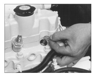
Figure 13: Remove and replace copper sealing washer.
