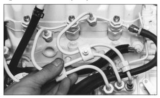
Figure 9: Remove delivery lines.
