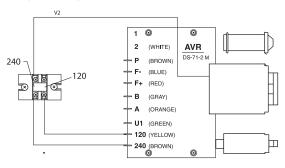
Figure 24: Control Terminal Board, 120/240 Volt Output
