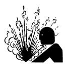
engine has been shut off. Do not remove a filler cap unless it is cool enough to comfortably grip with bare hands. Slowly loosen cap to relieve pressure before opening fully.
