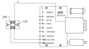
Figure 20: Control Terminal Board, 120 Volt Output
