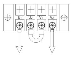
Figure 23: Output Terminal Board, 240 Volt Output
