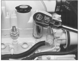
Figure 12: Unscrew injector.
