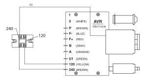
*Figure 22:* Control Terminal Board, 240 Volt Output b. Connect U2 to V1 on the output terminal board (Figure 23).
