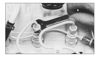
Figure 8: Remove delivery line flare nuts.
