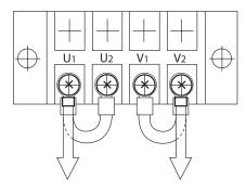
Figure 21: Output Terminal Board, 120 Volt Output
