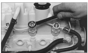
Figure 10: Remove return line nuts.
