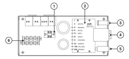
Figure 19: Control Box Components.
