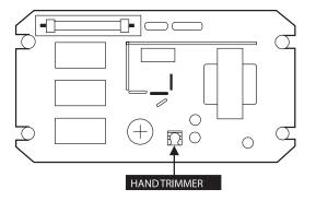
Figure 26: Hand Trimmer Location on AVR.
