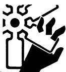
Wear close-fitting clothes. Stop the engine and be sure all fans, belts, pulleys and drives are stopped before making adjustments, connections, or cleaning near fans and their components.
