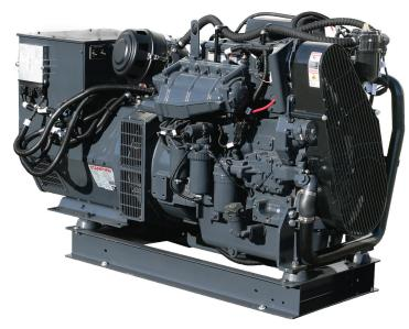
DC ELECTRICAL SYSTEM - Negative ground, 12 volt DC system includes starter motor and alternator with regulator. Low oil pressure and high coolant temperature safety shutdown system. Optional control panels help you specify the amount and type of information required. Comprehensive list of optional alarms and safety shutdowns. Optional DC logic system for simplified maintenance. Optional pre-wired engine, panel with terminal strips.
