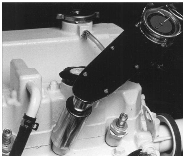
Figure 14: Reinstall injector. Torque to proper tightness.
