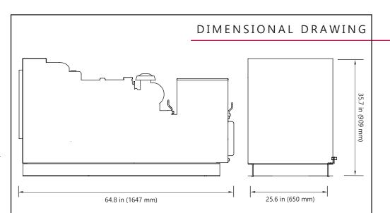
NL944D3 Overall Dimensions L x W x H: 64.8 x 25.6 x 35.7 inch (1647 x 650 x 909 mm) Dimensions given in inches (mm). Dimensions subject to change without notice. Contact dealer or visit www.northern-lights.com for most current installation drawings.
