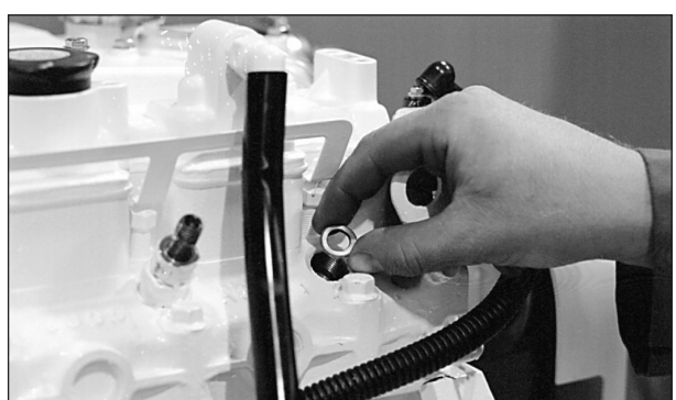
Figure 16: Remove and replace copper sealing washer.
