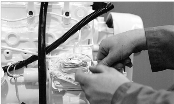
Figure 12: Cover lines, inlets and injection pump outlets.
