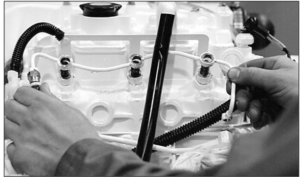
Figure 14: Remove return line.
