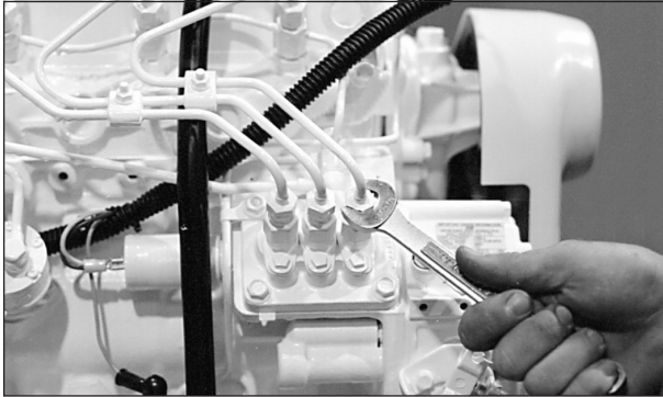
Figure 10: Remove delivery line flare nuts.
