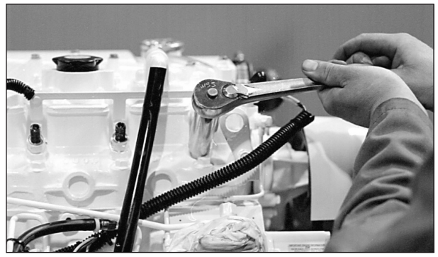
Figure 18: Reinstall injector. Torque to proper tightness.
