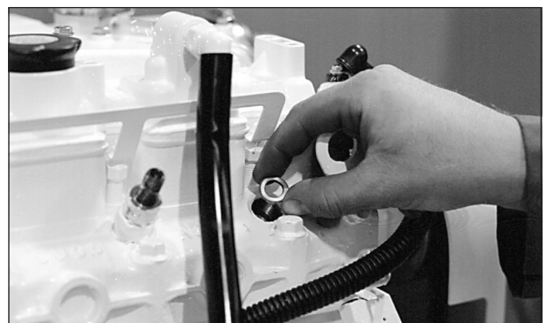
Figure 17: Remove and replace copper sealing washer.
