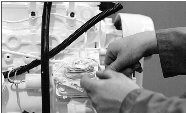
Figure 13: Cover lines, inlets and injection pump outlets.
