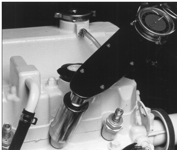
Figure 14: Reinstall injector. Torque to proper tightness.
