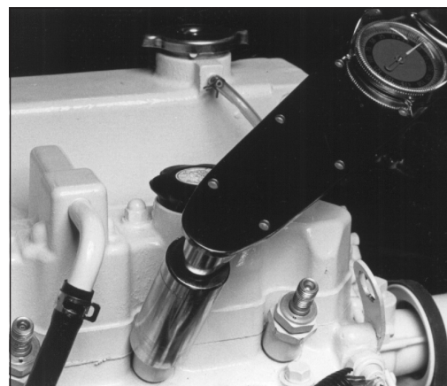
Figure 13: Reinstall injector. Torque to proper tightness.
