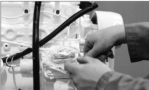
Figure 12: Cover lines, inlets and injection pump outlets.
