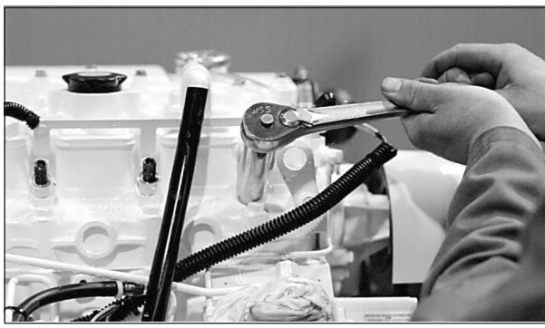
Figure 17: Reinstall injector. Torque to proper tightness.
