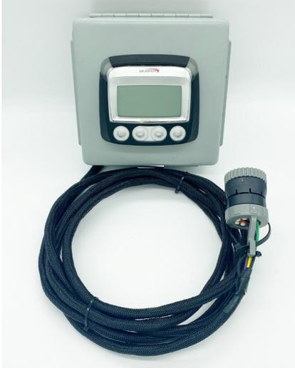
The PowerView display is a multifunction tool that enables equipment operators to view standard engine and transmission parameters and active/stored trouble codes. The display can show a single or a four parameter simultaneous display with text descriptions for most common fault conditions. The enhanced alarm indicators have ultra-bright alarm and shut-down LEDs.
