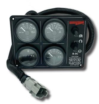
The S-3C is a flush mounted panel with manual start/ stop and engine monitoring analog gauges. The S-3C panel controls the engine pre-heat circuitry and the start/stop operations of Northern Lights Generator.
