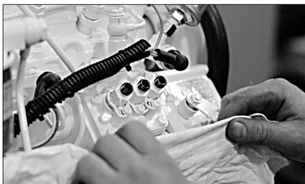
Figure 15: Cover lines, inlets and injection pump outlets.
