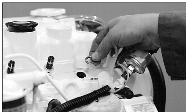
Figure 19: Remove and replace copper sealing washer.
