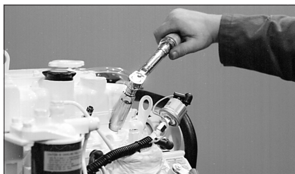
Figure 20: Reinstall injector. Torque to proper tightness.
