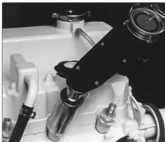
Figure 16: Reinstall injector. Torque to proper tightness.
