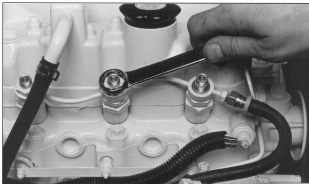
Figure 12: Remove return line nuts.
