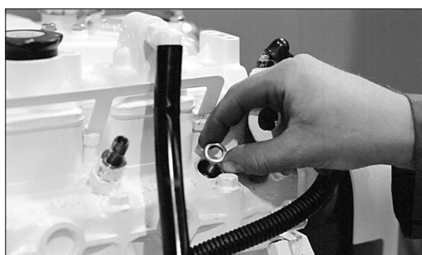
Figure 17: Remove and replace copper sealing washer.
