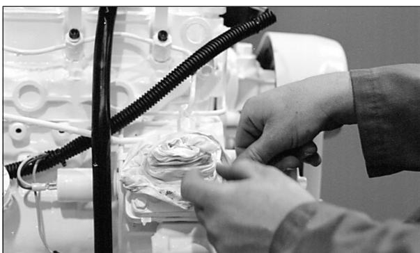
Figure 13: Cover lines, inlets and injection pump outlets.
