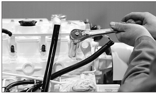
Figure 18: Reinstall injector. Torque to proper tightness.
