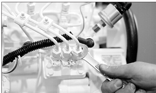
Figure 7: Remove delivery line flare nuts.
