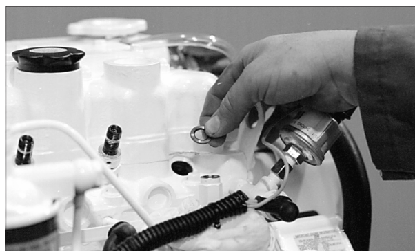
Figure 13: Remove and replace copper sealing washer.
