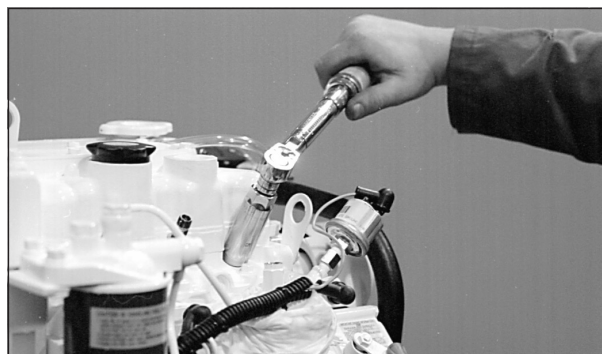
Figure 20: Reinstall injector. Torque to proper tightness.
