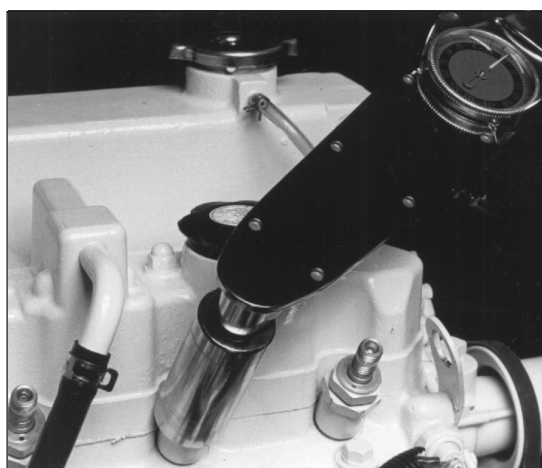
Figure 16: Reinstall injector. Torque to proper tightness.
