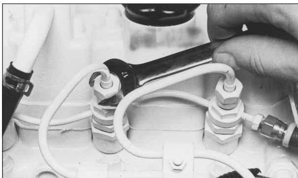
Figure 10: Remove delivery line flare nuts.
