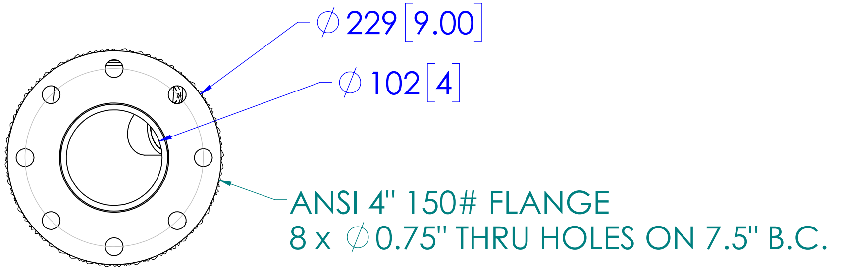
DETAIL A OPTIONAL DRY EXHAUST FLANGE SCALE 1 : 4
