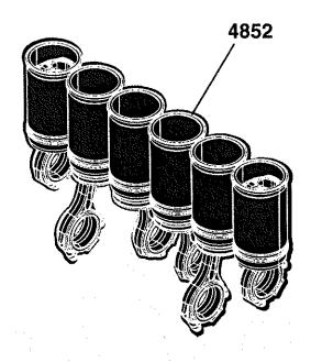
4852 Connecting Rod, Piston and Liner 4852 Bielle, piston et chemise 4852 Pleuelstange, Kolben und Büchse 4852 Biella, pistone e camicia 4852 Biela, émbolo y forro 4852 Vevstake, kolv och foder
