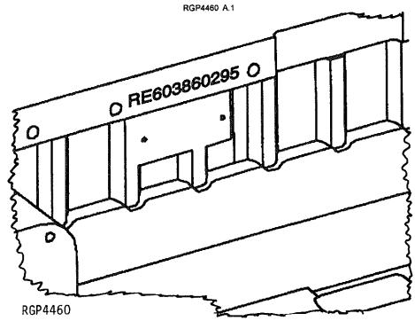
Serial number stamped into casting of block near previous serial number plate.
