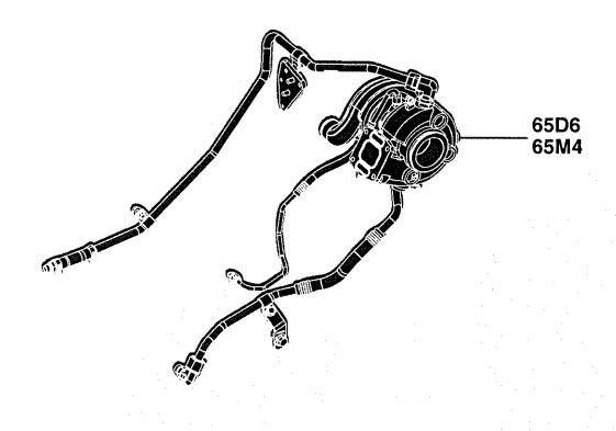
65D6 Turbocharger 65D6 Turbocompresseur 65D6 Turbolader 65D6 Turbocompressore 65D6 Turbocompresor 65D6 Turboaggregat 65D6\_RE547118\_PCD A.1
